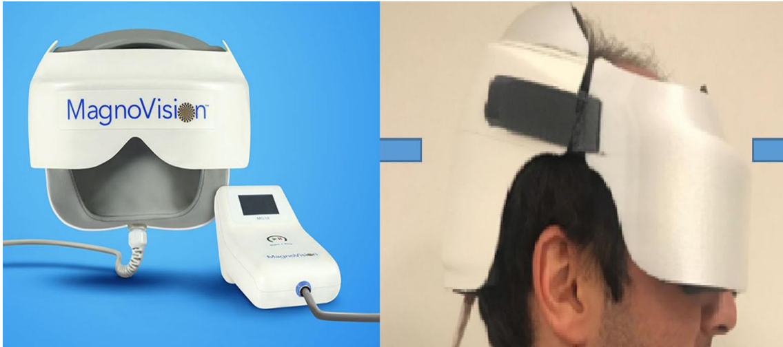
Figure 3: Retinal electromagnetic stimulator (rEMS) device. Application of the helmet to stimulate the retina-optic nerve and visual pathways.
